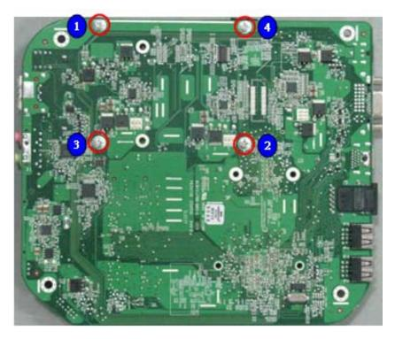
2. Remove HDD from Main board.
